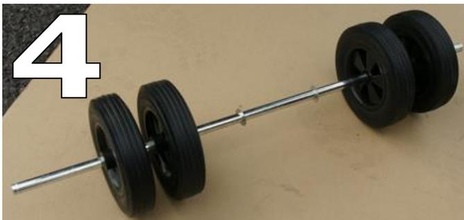
4. Prepare the rear fixed wheels as shown, NOTE the two washers in the middle. Don't use any C clips just yet
