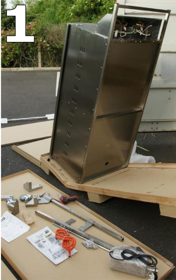
1. Lay out all your components on a cushioned surface. Put the oven on its end and attach the wheels. Start with the castor wheels at the burner control end
