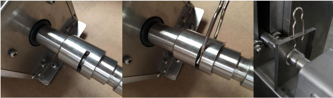
Familiarise yourself with the spit to motor connector and be careful not to lose the U shaped pin, (U Clip). You will find two holes on the motor bracket where this pin can be stored when not in use.
