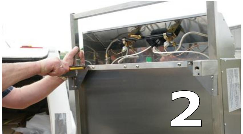
2. Tighten these into place using the bolts and spanner provided.
