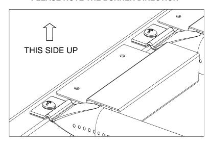
Inspect burner for any damage (cracks or holes). If damage is found, replace with a new burner. Reinstall the burner, check to ensure that the Gas valve orifices are correctly positioned and secured inside the burner inlet (venturi).
