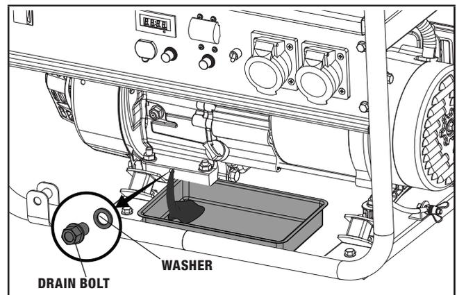
3. Replace the oil drain bolt and washer.
