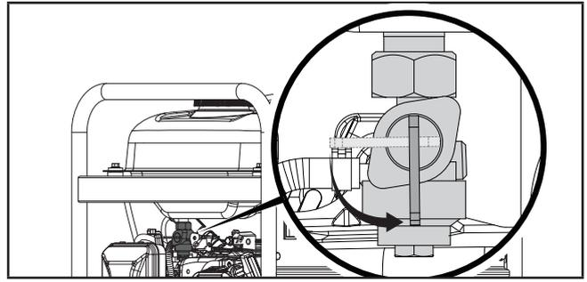
4. Push the engine switch to the "ON" position.
