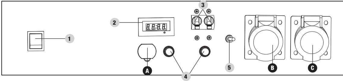
1. **Engine Switch** – Used to put in START mode or STOP the generator.
