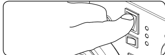
7. **ELECTRIC START:** Press and hold the ignition switch to the "START" position. Release as the engine begins to roll over. If the engine fails to start within five seconds, release the switch and wait at least ten seconds before attempting to start the engine again.
