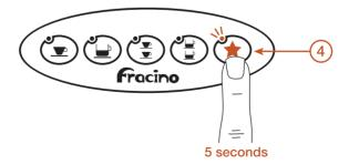
**4)** Press the star button on the left hand touch pad and hold for 5 seconds until the lights above the symbols start to flash. The machine is now in program mode.
