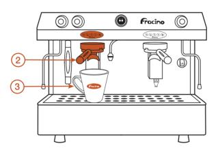
2) Put one shot of coffee into a single filter holder and fit the holder into the left hand group as shown at the start of this section. 3) Put the espresso cup under the beak,
