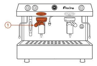
1) Machines with two or more groups are programmed on the left hand group/touch pad. When the process is completed the settings will be stored for all groups. Any groups to the right can be programmed independently by following the same procedure.
