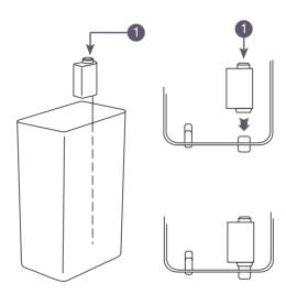
2) Fill the water tank with fresh cold water, this can be done with a jug. Alternatively the tank can be removed and filled at a sink.
