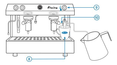
8) Place the cup you are using to make your chosen drink under the frother nozzle. 9) Open the steam valve to push steam through the frother. 10) When you have got the required amount of frothed milk close the steam valve.
