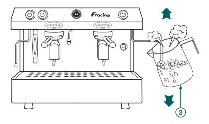
3) Move the jug gently up and down so that the tip of the steam nozzle is in the top 25mm of the milk to incorporate air into the milk and to create a froth. As the milk foams move the jug up to heat the milk.
