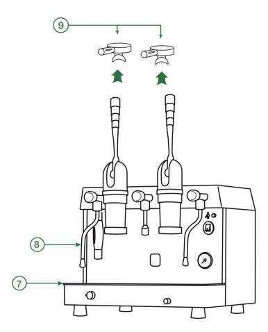
7) Lift out the outer and inner drip tray. Clean both sides in warm soapy water. Do not use a scouring pad.
