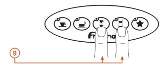
9) Re-setting the counter can be done by pressing the double espresso and double cappuccino buttons simultaneously. The display will read "RESET H2O FILTER COUNTER...WAIT". The display will return to "SELECT DRINK FRACINO".
