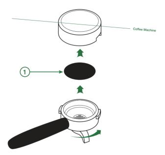
1) Romano coffee machines have a unique automatic cleaning cycle programme in the electronics enabling the operator to place the blank filter into each group in turn.
