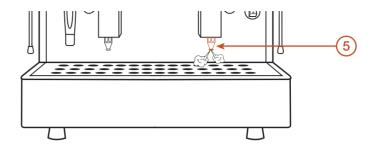
5) Press the button to start the coffee flow as shown below. Once the coffee flow stops any excess pressure that is left in the filter holder is discharged through the exhaust valve below the group. Remove the filter holder from the group, empty used coffee grounds into drawer or receptacle and place empty filter holder back in the group to keep it warm.
