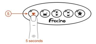
5) Press the single espresso button within 5 seconds and allow the coffee to fill the cup to the required level. Press the button again to stop and store the setting.
