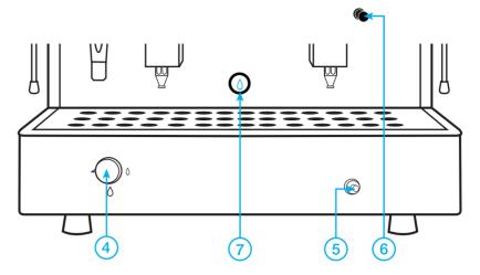
4) To ignite the burner turn the main gas regulator/isolation valve on. 5) Press the silver gas flow control valve button in and hold. 6) Press the black electronic ignitor button until a blue flame appears. 7) This can be viewed through round hole in front panel. Keep the silver gas flow button depressed for 20 seconds to allow thermocouple to reach temperature then release slowly.
