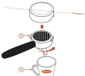
3) Put the filter holder into group. It will fit into the group from the left and turns to the right until the handle is facing forwards towards you. 4) Place the warmed cup(s) under the filter holders and in line with the beak(s).
