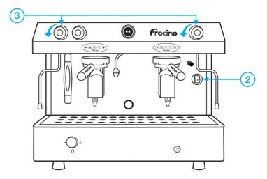
2) Switch the machine on via the on/off switch. 3) Open the steam valve to allow the air to vent.
