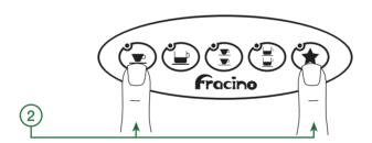
2) The cleaning function is enabled by pressing the star button and holding and simultaneously pressing the espresso button.
