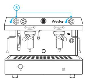
8) Once steam starts to pass through the steam tube (approximately 15 minutes using electricity or 30 minutes using gas from switching machine on) close the valve. The pressure will be then build up to 1.0 - 1.2 BAR.
