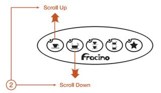
2) Press the espresso button to scroll up through the buttons and the cappuccino button to scroll down.
