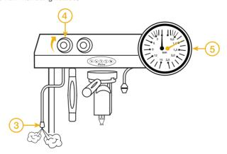
3) Once steam starts to pass through the steam tube (approximately 15 minutes from switching machine on). 4) Close the valve(s). 5) The pressure will then build up to 1.0 Bar.
