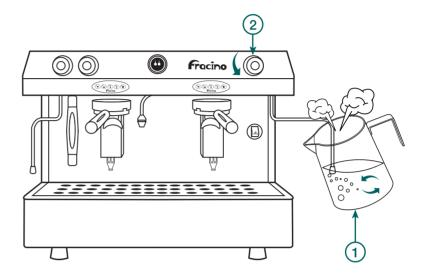
1) Fill 1/3 of a jug with fresh cold milk. Then insert the steam tube into the milk with the nozzle below the surface of milk. 2) Fully open the steam valve. Place the steam tube to the front of the jug to help the milk circulate and froth.
