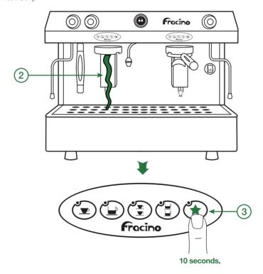
2) Remove the filter holders from the groups. 3) Press the star button to allow water to flow freely for approximately 10 seconds.
