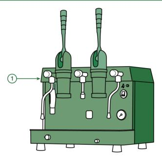
1) Wipe the outer casing of the machine with a soft damp cloth (do not use a scouring pad). Use a shower plate brush, soaked in to some liquid quartz, to dislodge dried coffee particles in the group and around the filter holder washer to prevent a build up of coffee. (Brushes can be obtained from Fracino, part no.FC54
