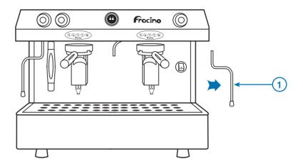
1) Make sure the machine is off and has cooled down sufficiently then remove either the left or right steam tube depending on which side you prefer to attach the Rapido Idea frother and attach the short steam tube in place of the standard tube.
