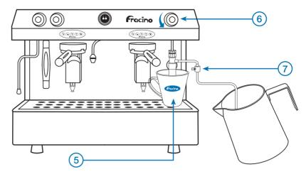
5) Place the cup you are using to make your chosen drink under the frother nozzle. 6) Open the steam valve to push steam through the frother. 7) Gently wind the milk regulator screw attached to the rubber tube outwards to draw milk up the tube into the frother which will then froth the milk into the cup. When you have got the required amount of frothed milk turn off the steam valve.
