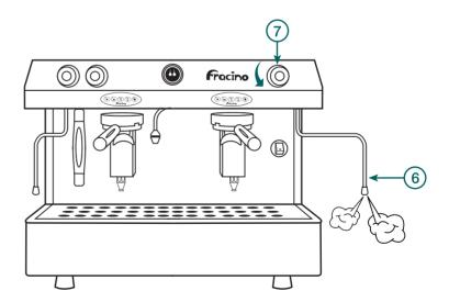
**6)** Wipe the steam tube with a damp cloth to remove milk residue. **7)** Open the steam valve to clear any remaining milk from the tube/nozzle. Periodically remove the nozzle and clean with warm water ensuring the holes are clear (this can be done with a bent paper clip).
