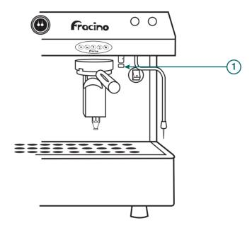
When the Cappuccino mode is selected, the amount of air entering the system can be adjusted. This is so that the consistency of the frothed milk can be adjusted.
