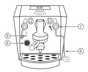
6) Wait for steam to vent from the steam tube (which will take between approximately three and four minutes). 7) Then close the steam valve by turning the black handle clockwise until it stops.
