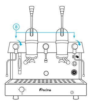
8) Once steam starts to pass through the steam tube (approximately 15 minutes using electricity or 30 minutes using gas from switching machine on) close the valve. The pressure will be then build up to 1.0 - 1.2 BAR.
