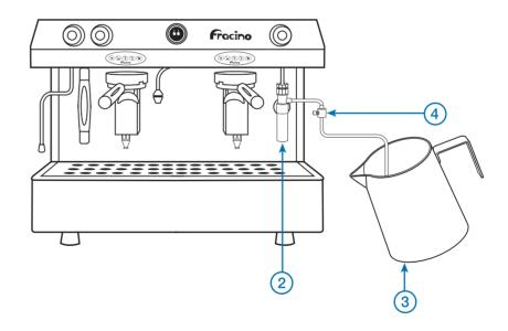
2) Carefully attach the the Idea Rapido frother in place of the removed steam tube taking care not to overtighten 3) Place the long rubber tube attached to the side of the frother into a jug of your chosen milk. 4) Make sure the screw on the milk regulator is fully screwed in before turning the machine back on. Please then follow the machine start up procedure.
