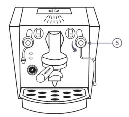
5) Open the steam valve by turning the black handle anti-clockwise.
