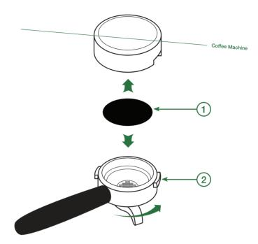
Now the groups must be backwashed. 1) This is done by inserting the blank filter into one of the filter holders. 2) Then put the filter holder into one of the groups as if making coffee.
