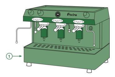
1) Wipe the outer casing of the machine with a soft damp cloth (do not use a scouring pad). Use a shower plate brush to dislodge dried coffee particles in the group and around the filter holder washer to prevent a build up of coffee. (brushes can be obtained from Fracino, part no. FC54).
