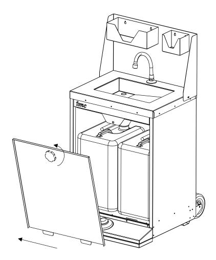
Once the front panel has been removed, lift out the suction hose from the clean water container and remove the water container. Note the water container can hold a maximum of 20 litres. You can fill the container with less if you want. Ensure when refitting the water container that the suction hose has been placed at the bottom container. Check that the funnel is fitted to the waste container and position under the sink waste pipe.
