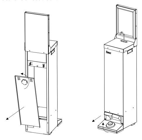
Once the rear panel has been removed, fit the suction hose pipe into the sanitiser container. Place the container on to the inner base panel. Note the suction tube is suitable for 5 litre containers.
