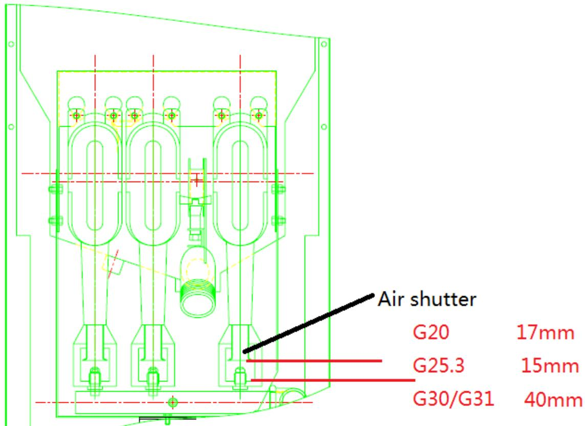
Unscrew the locking screw of the burner air shutter and adjust the air shutter to desired height. In the above picture you can find the suggested height for different types of gases. The height is the distance between burner base and air shutter.
